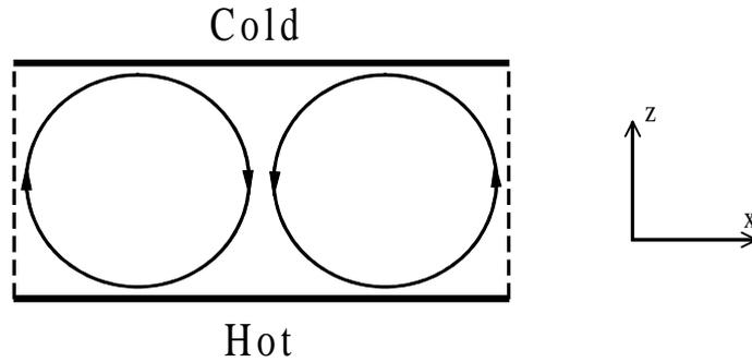
Figure 1.1: The physical system modelled by Lorenz
